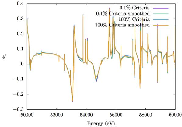
Fig. 1. Coefficient of first moment in Legendre expansion of angular distribution of elastic scattering for  $^{63}\text{Cu}$  in RRR for the 0.1% and the 100% relative error in the linear interpolation criteria, with smoothed versions.
