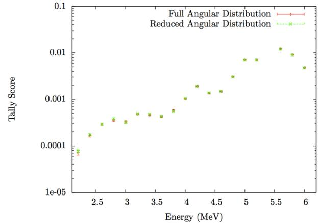
Fig. 3. Tally results for calculated neutron current across one face of a cube model filled with  $^{16}\text{O}$  binned versus energy.
