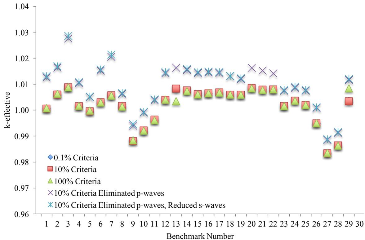
Fig. 4.  $k_{\text{eff}}$  results for the set of 29 benchmarks described in Table IV for four different reductions of the number of energy points used to describe the angular distributions of elastic scattering for the two isotopes of copper. (The stochastic uncertainty on the calculations is below 10 pcm, which is smaller than the size of the markers.)
