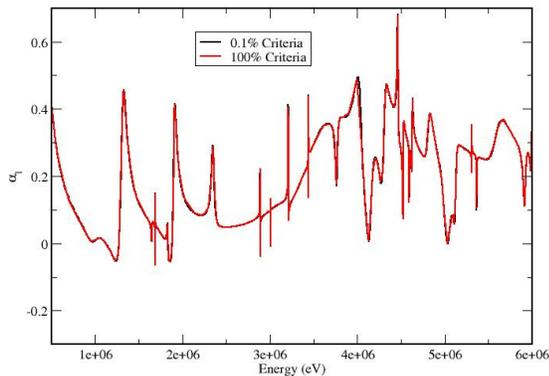
Fig. 2. Coefficient of first moment in Legendre expansion of angular distribution of elastic scattering for  $^{16}\text{O}$  in RRR for the 0.1% and the 100% relative error in the energy range 500 keV and 6 MeV.
