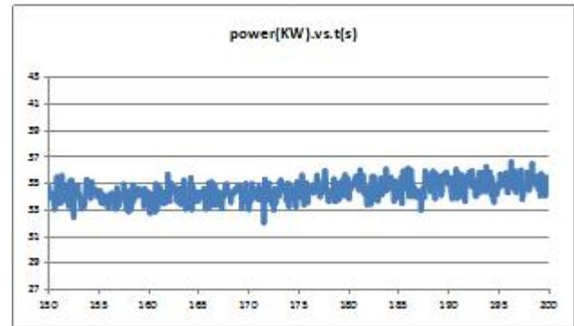
Figure. 4. The calculated power history of TRACY by the TCCAHR with oscillations model
