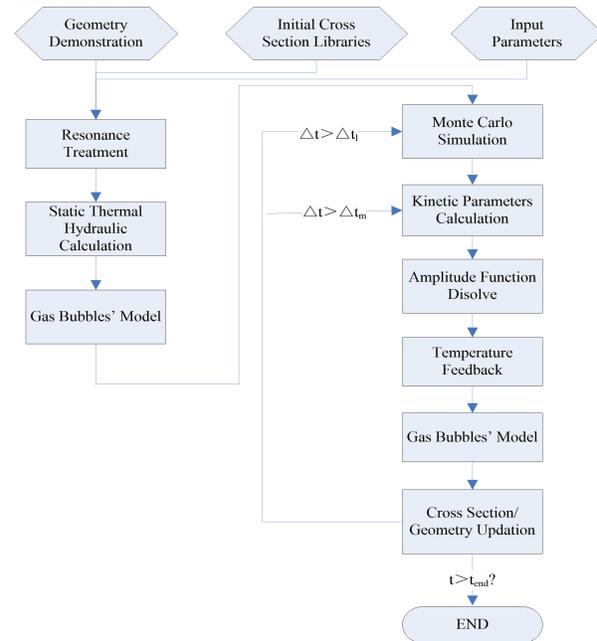
Fig. 2. Flow Chart of TCCAHR with Gas Bubbles' Model
