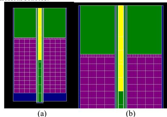
Figure. 1. Geometry consider of TRACY((a)Right view of geometry description of TRACY; (b)Small fuel regions in the free surface)
