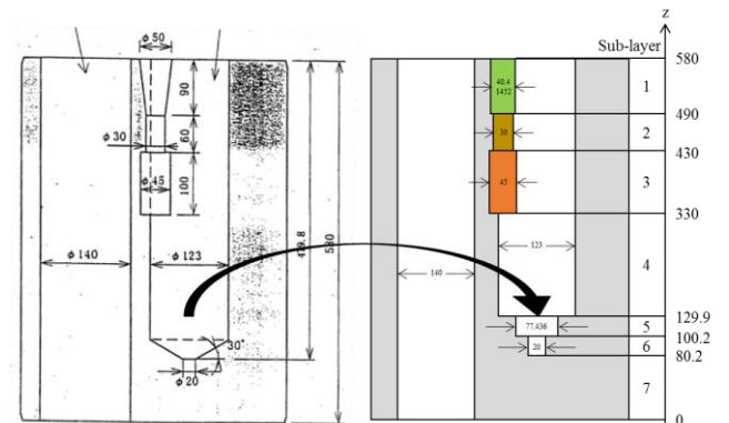
Fig. 6. Approximation of the RSS insertion hole in control rod guide block at 7 th layer.
