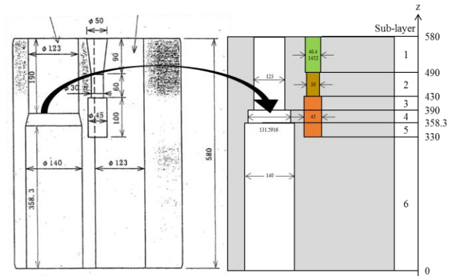
Fig. 5. Approximation of the control rod insertion hole in control rod guide block at 6 th layer.
