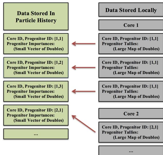
Fig. 2. Progenitor Tallies are stored locally and Progenitor Importance and unique identifier information are communicated to the Master Node.
