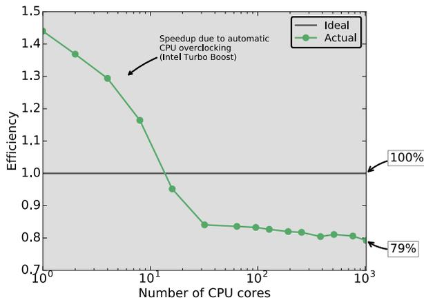
Fig. 3. Efficiency of parallel GPT sensitivity calculations. The greater than 100% efficiency occurs for simulations
