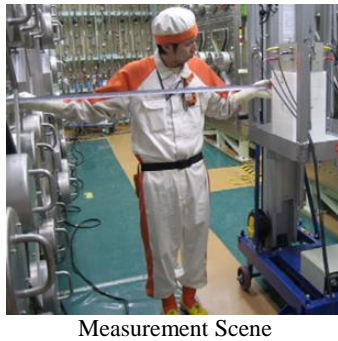
Fig.2. A hand-held neutron detector for BCAT and measurement scene
