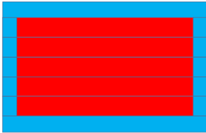
Fig. 2: Illustration of a simple core model formed from two slice types. One slice type would represent the top/bottom reflectors (blue) and another slice type would represent the active core (red) plus radial reflector (blue). The composite model is formed as a stack of the slice types.
