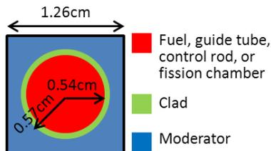
Fig. 8. Pin-cell of the modified 3D C5G7 problem
