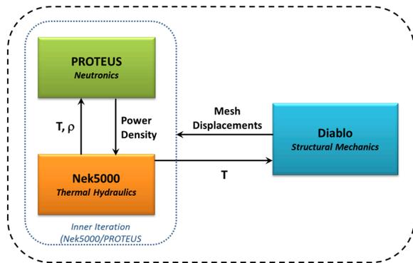
Fig. 2. Schematic of the SHARP Toolkit Workflow for Modeling Core Deformation.
