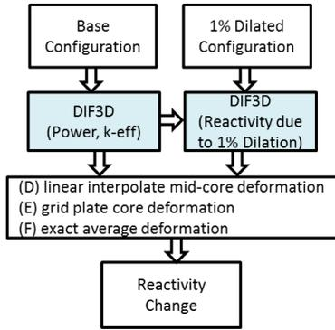
Fig. 6. Method D, E, F Workflows: Emulates SAS4A/SASSYS-1 Simple Method, Grid Plate Expansion-Only, and new Hybrid Method.
