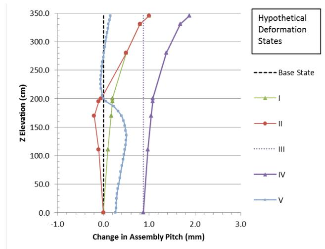
Fig. 8. Hypothetical Radial Core Deformation States Applied for ABTR Analysis.
