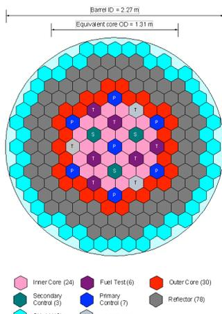
Fig. 7. Core Map of the Advanced Burner Test Reactor.
