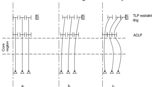
Fig. 1. Deformation States for a Limited Free Bow Restraint System showing a) Undeformed State, (b) Intermediate Deformation State, (c) Limited Free Bow State.
