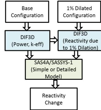
Fig. 4. DIF3D/SE2-ANL/PERSENT/NUBOW-3D Calculation of Core Deformation Reactivity Feedback
