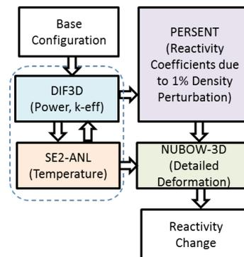
Fig. 3. DIF3D/SE2-ANL/PERSENT/NUBOW-3D Calculation of Core Deformation Reactivity Feedback.
