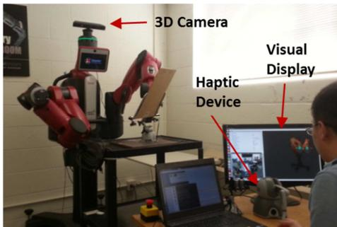
Fig.6. Augmented Teleoperation Testbed
