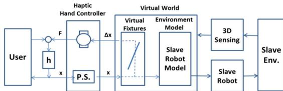
Fig.5. Augmented Teleoperation System Architecture
