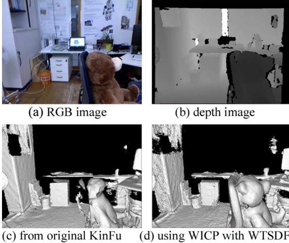
Fig.3. Comparison of 3D reconstruction of “Teddy” at the 400th frame
