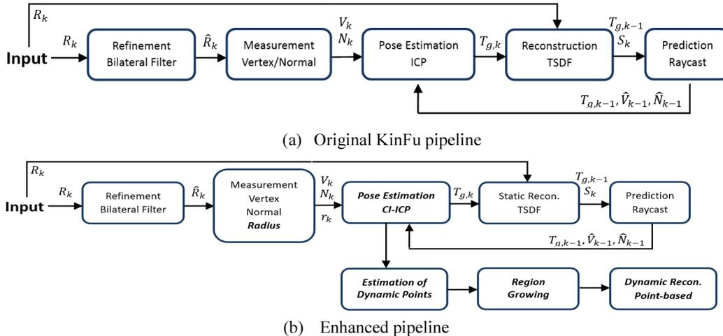
Fig.2. Real-time 3D Reconstruction Pipeline
