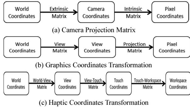
Fig.7. View Perspective Transformations for Visual-Haptic Rendering
