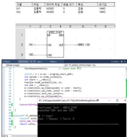
Fig.6 An example of function block testing of test-bed.
