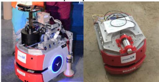
Fig 1. Radiation Survey System<sup>[1]</sup>. Configured to sweep floors for alpha contamination (left) or for beta/gamma detection as presented in this paper (right).
