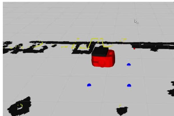
Fig 6. The RViz-based GUI allows the user to rotate the real-time updates from the system to any desired 3D perspective. Note also that the real-time obstacle data (yellow) is layered on the original map (black)
