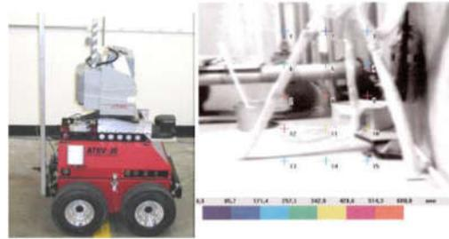
Fig 2. INL Mobile Radiation Surveying Platform and Data Display [9]
