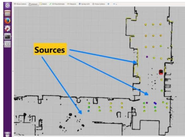
Figure 10. Map produced by the robot. Dots are color coded by radiation intensity. Violet is the strongest readings with higher wavelength colors for lower readings.
