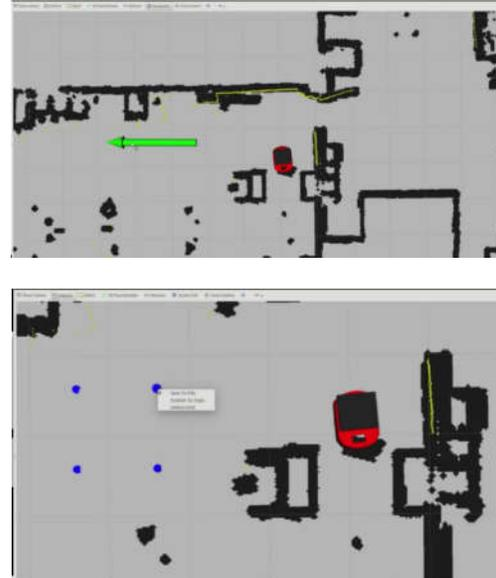
Fig 5. Survey Grid Tool. The user places the grid origin with an arrow (top). After adjustments, send the survey plan to the robot or save to file (bottom). Once the grid is place, it can easily be selected and then translated or rotated in the mapped space before the user saves the proposed survey.
