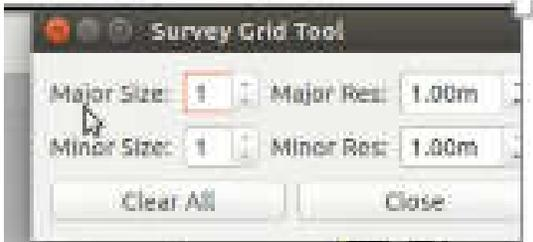
Fig 4. Pop-up in survey generation system used by operator to define grid size and resolution.
