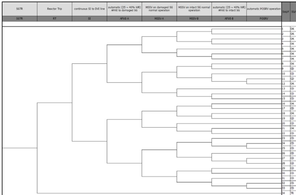
Fig.1 ET of SGTR considering the status of safety valves
