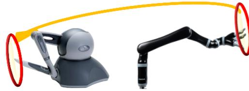
Fig. 11 Applying a manipulability ellipsoid from the slave robot to the master device.
