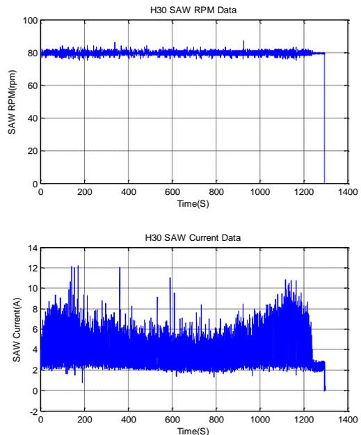
Fig. 6 Control responses of cutting motor.
