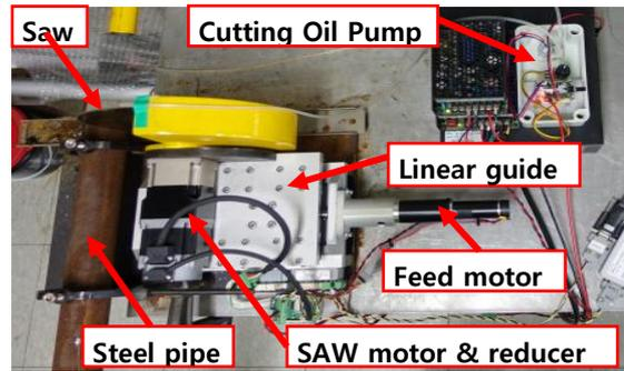
Fig. 5 Cutting tool test bed.
