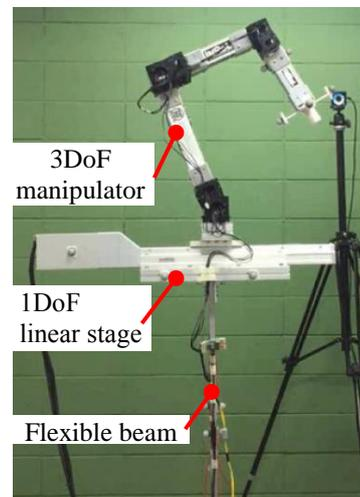
Fig. 13 A shared control test bed of the manipulator on the flexible base.
