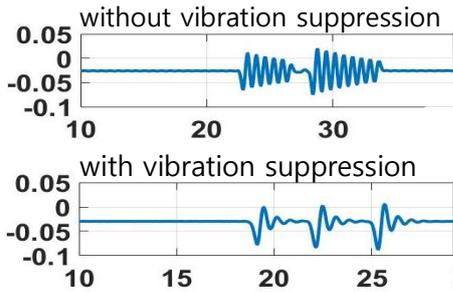
Fig. 14 Vibration suppression control response.
