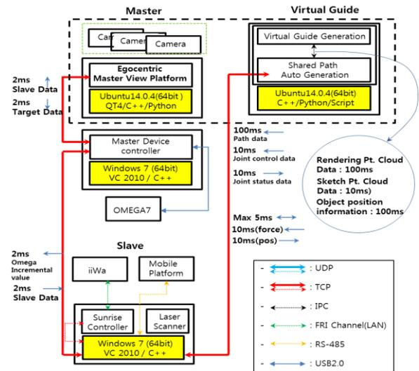
Fig. 11 Software integration diagram
