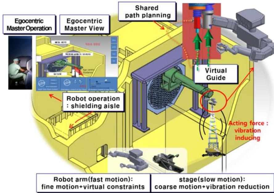
Fig. 2 Concept of maintenance tasks in nuclear facilities.
