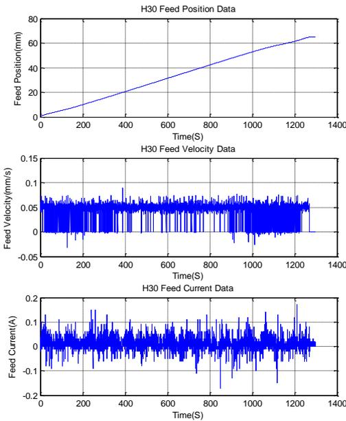
Fig. 7 Control responses of feeding motor.
