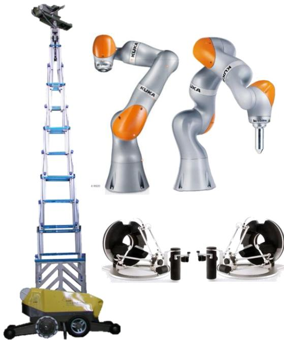
Fig. 3 Mobile platform, slave and master.
