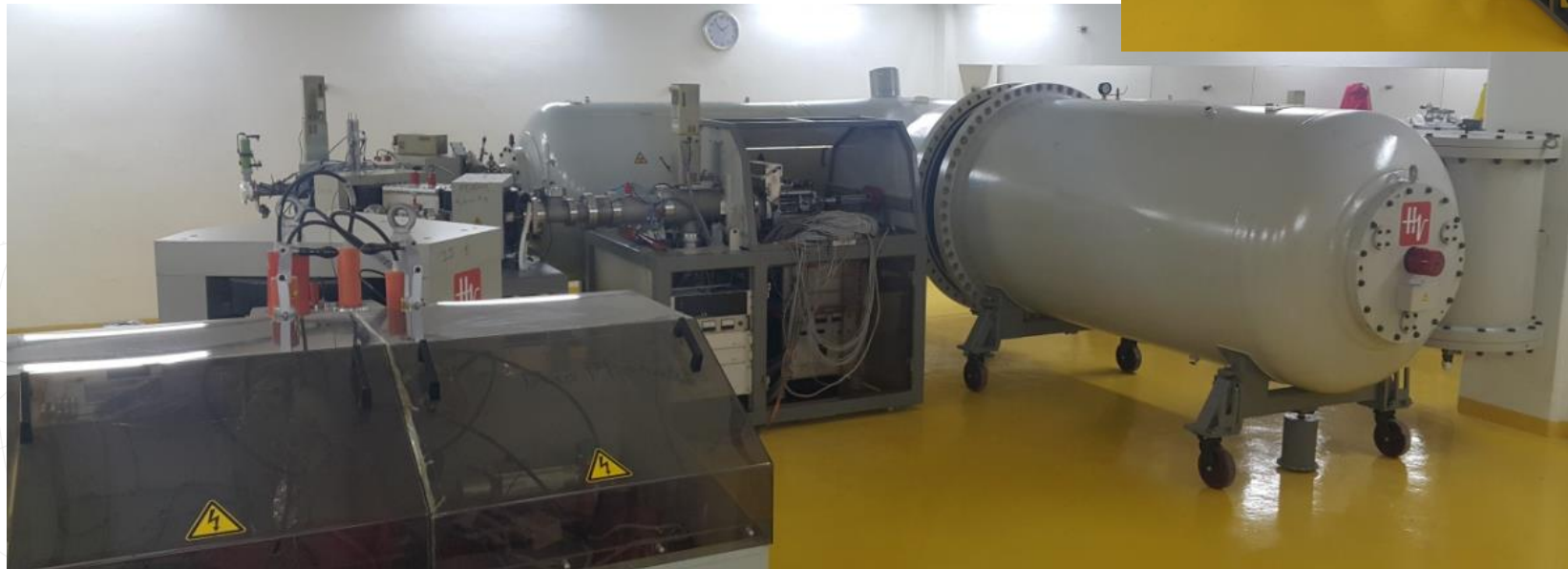
3 MV Tandem under installation
