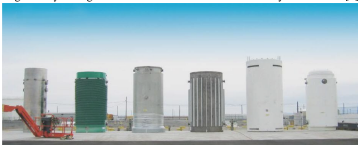
Figure. Dry Storage Casks at the Idaho National Laboratory INTEC Site [1]
