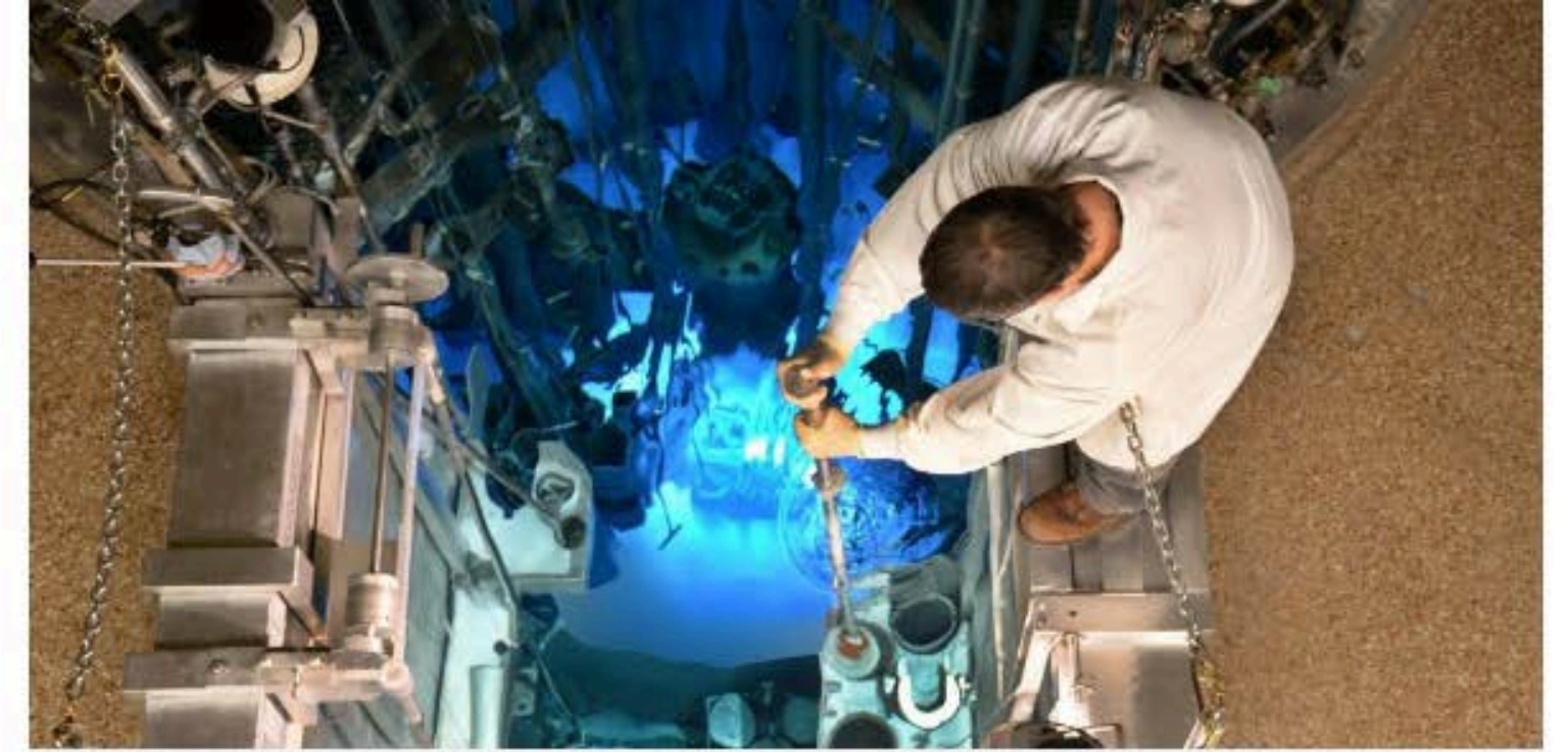
A reactor operator retrieves a sample can from the MURR, as seen from above. (Photo: University of Missouri)
