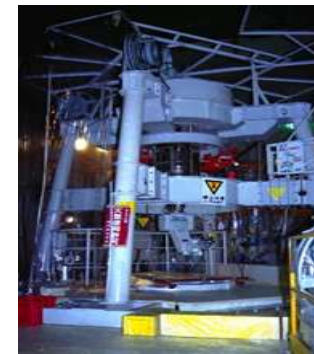
<Robotic manipulator cutting device>
