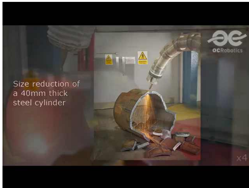
<40 mm thick steel cylinder Cutting (x4)>
