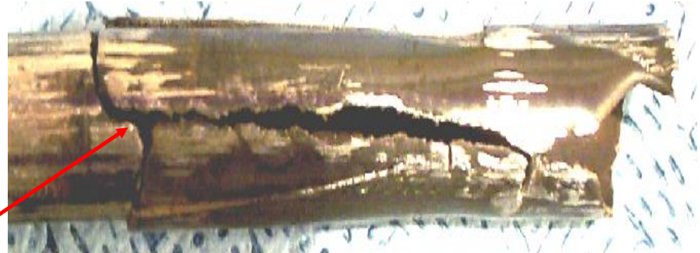
[SCC and Rupture of U-4 SG Tube]
