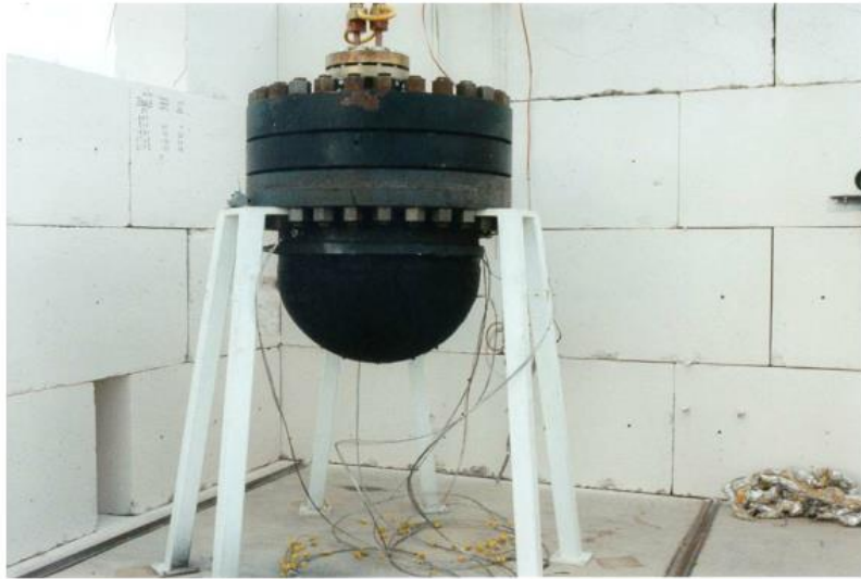
Figure 2.9 Assembled vessel on test stand
