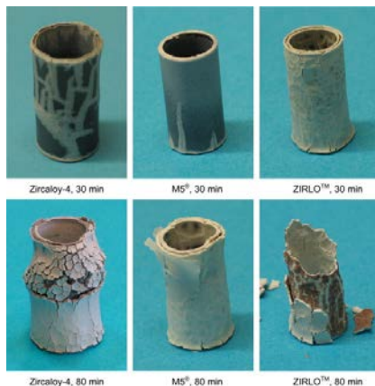
(Left) High-temperature oxidation behavior of zirconium alloy cladding, (right) Picture of a nuclear accident with hydrogen explosion after LOCA
