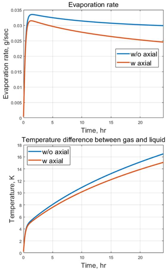
Fig. 6. Evaporation rate and temperature difference between gas and liquid with respect to time.
