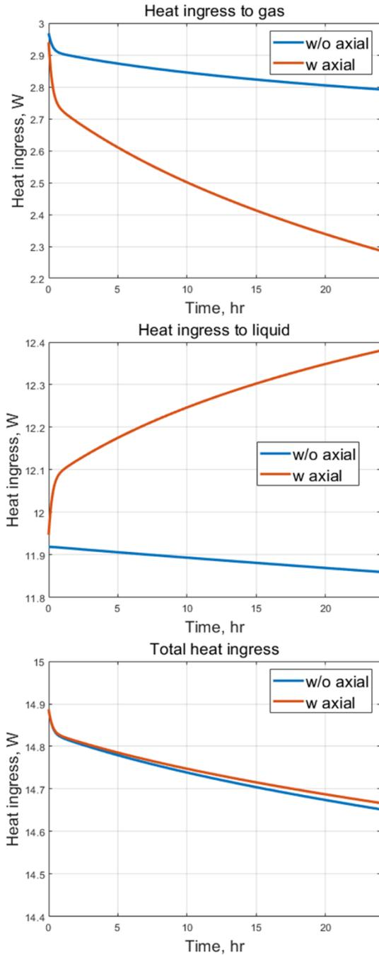
Fig. 4. Heat ingress to gas, liquid, and total.
