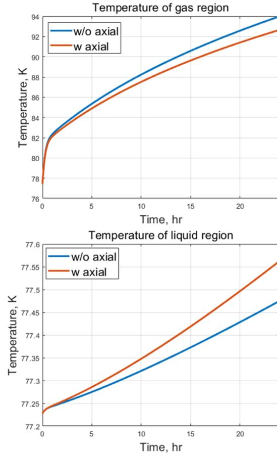
Fig. 5. Temperature of liquid and vapor region with respect to time.
