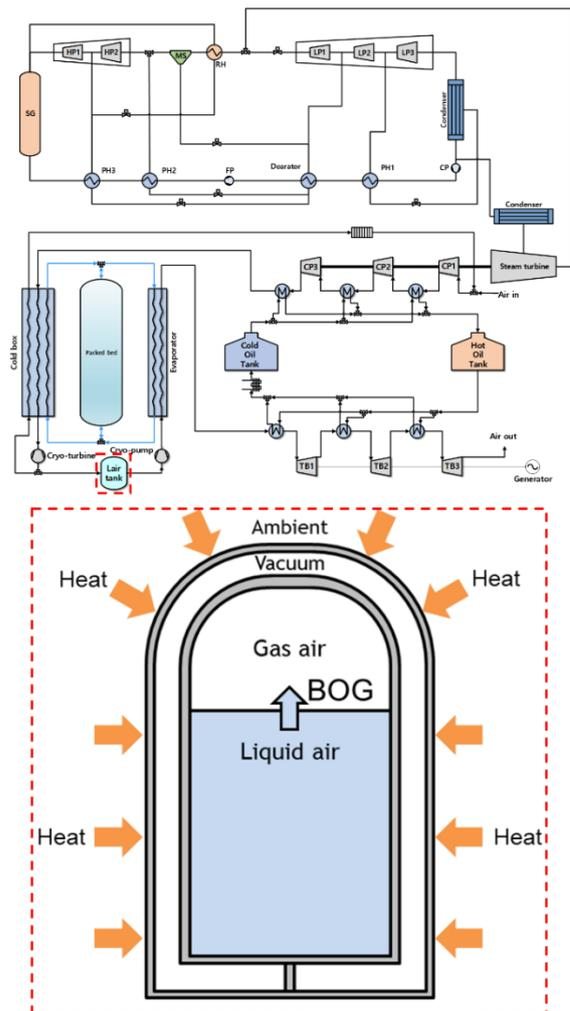
Fig. 1. Schematic diagram of liquid air energy storage system
