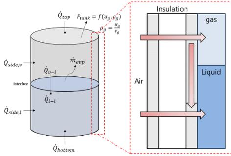
Fig. 2. Schematic diagram of liquid air tank and side wall.
