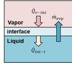
Fig. 3. Heat transfer at the interface.
